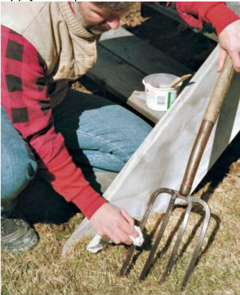
Oil steel tool heads to prevent them from oxidizing. The oil creates a barrier between the air and the steel.
