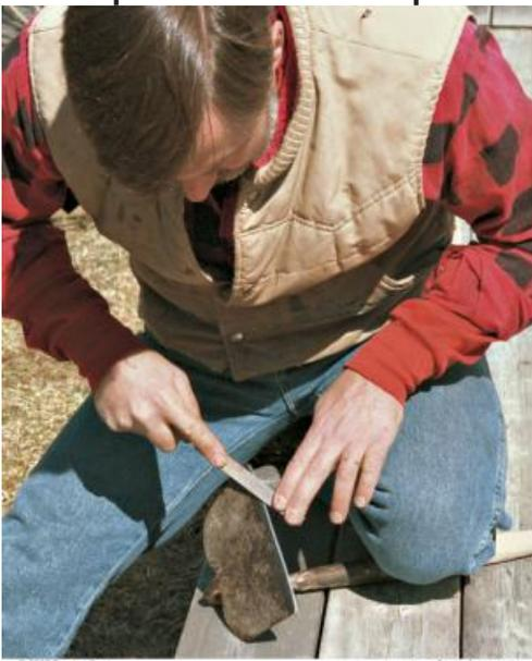
Use a hand-held mill file to sharpen hoes and shovels. The key to successful sharpening is keeping the tool steady and the file at the proper angle.
