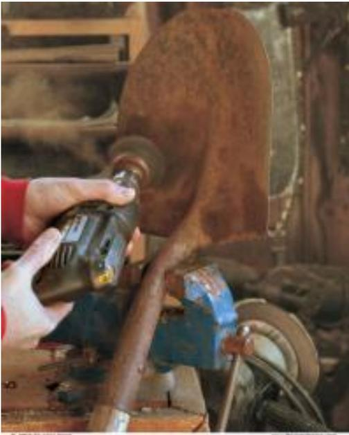
For a very heavy coat of rust, use a drill with a wire brush attachment
