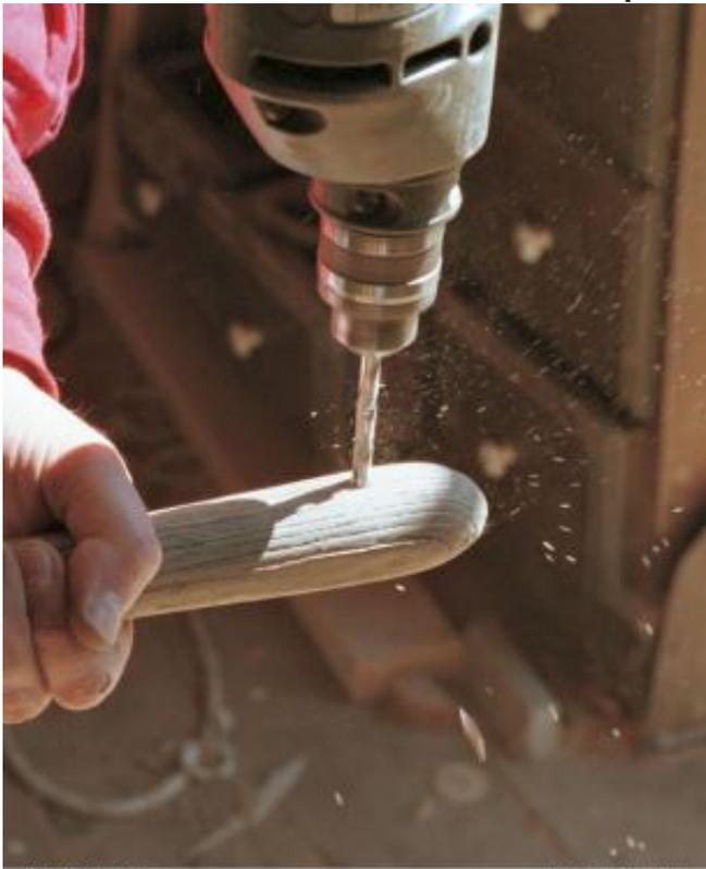
Drill holes in tool handles so they can be easily hung from nails affixed to the walls of a garage or storage shed.
